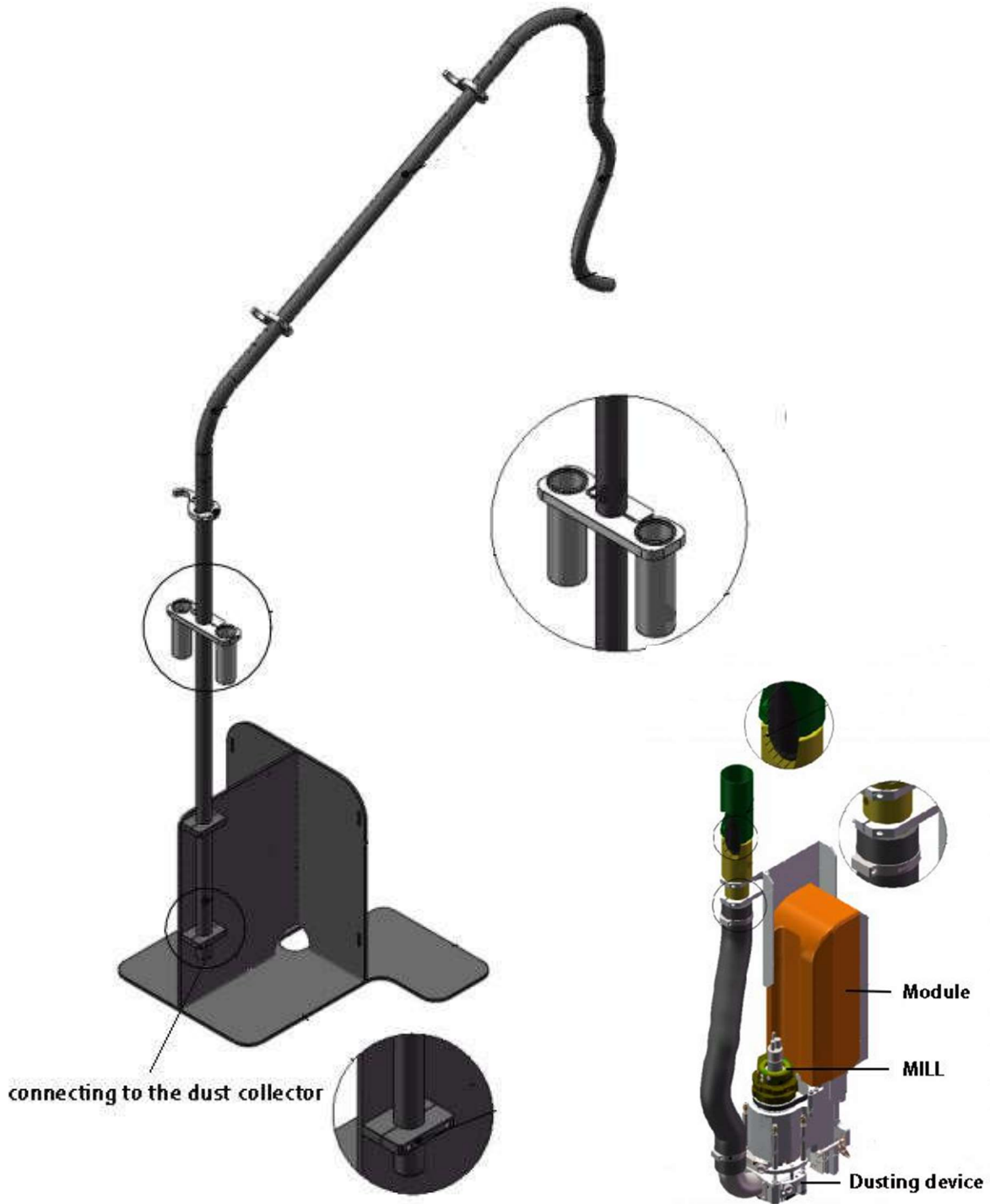
3.5.1 Connect cables in the milling device support
